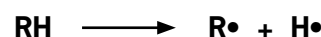
Figure 1 - Initiation phase: Oxidation at a double bond (RH) gives a free radical (R•) and a hydrogen atom (H•)
